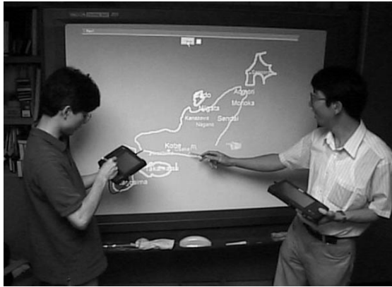
Figure 2: A digital whiteboard system using the multiple-device architecture. Note that two users are simultaneously using the same whiteboard, maintaining personal application states in their palmtops.
