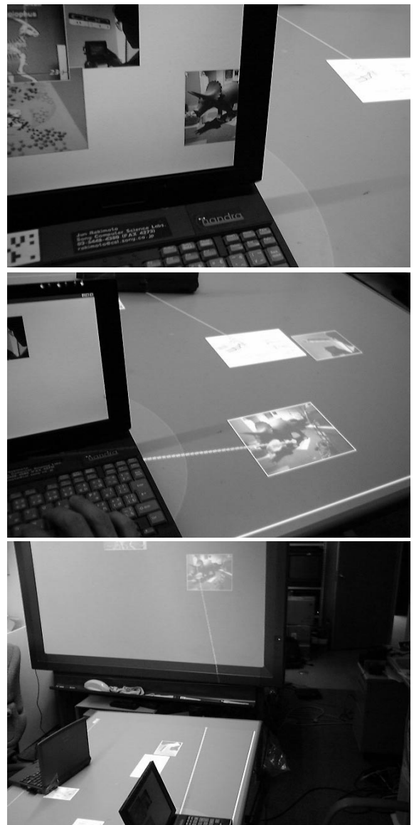
Figure 4: Moving information using "hyperdragging": A user can drag-and-drop a digital object between a notebook PC and a table surface display. During its operation, an "anchored cursor" line connecting the cursor and the notebook appears on the table display.
