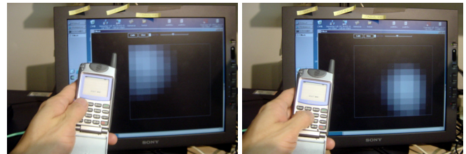
Figure 1: A cellular phone keypad with an embedded SmartPad sensor. The recognized finger position appears on the screen.
