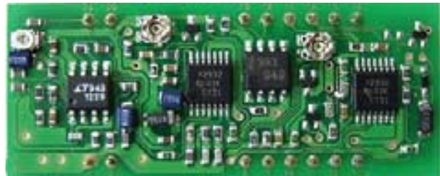
Figure 5: TouchNet Module: The module size is 20×48 mm and can be put into a wearable key and ubiquitous keyholes. The transmission speed is 9600 bps, and the module has half-duplex communication.
