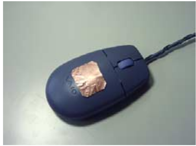
Figure 9: Ubiquitous Keyhole: The TouchNet module is installed in the PC's mouse as a keyhole and connected to the PC through an RS-232C interface. The electrode of the TouchNet module is placed on top of the mouse.
