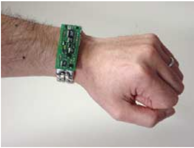
Figure 8: Wearable Key: The TouchNet module is put into a wristwatch-like unit. The user wears the key with the electrode of the TouchNet module in contact with the body.
