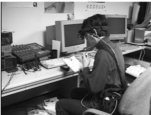
Figure 5: Wearable system is used to attach a voice note to the physical object
