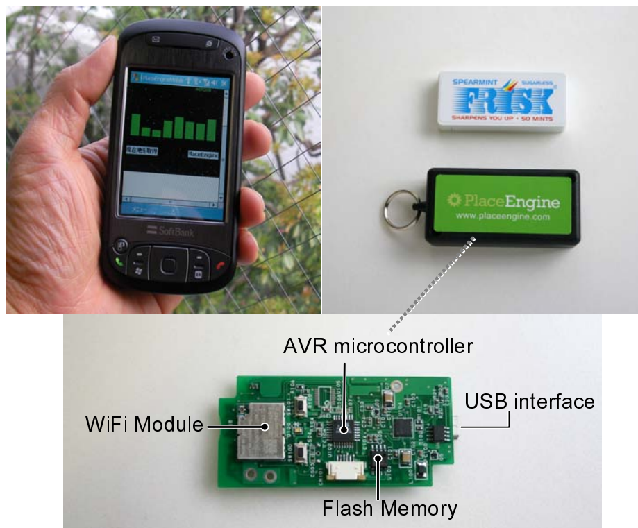
Fig. 5. LifeTag: two hardware configurations (left: smart phone version, right: keychain version with custom logging hardware)
