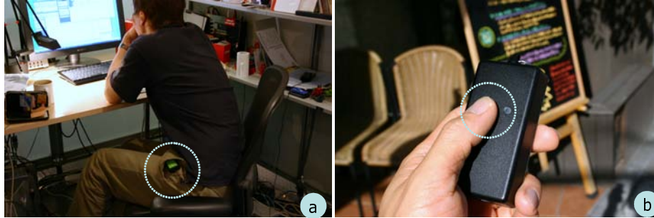
Fig. 7. Using LifeTag on a daily basis: (a) continuously logging locations in indoor and outdoor environments. (b) manually bookmarking a place of interest.
