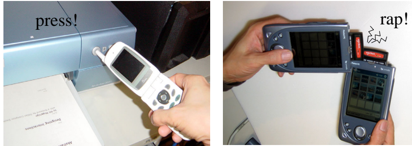
Fig. 10. Variations of SyncTap operations (left: a button of one device is used to "press" the other device's SyncTap button, Right: knocking on the device with the other device, causes synchronously generated sound.
