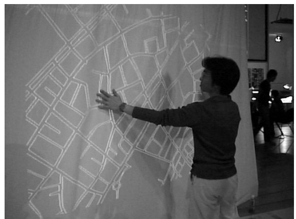
Figure 5: A Map browser on a curtain: When a user touches a map projected on a curtain with one or two hands and moves hands in the same direction, the map moves according to the hand movement. A user can also expand or shrink the map by controlling the distance between two hands.
