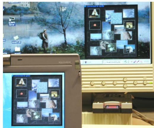
Figure 15. transGate: These two PCs access to the “same” shared space in tranSticks (not in a server)
