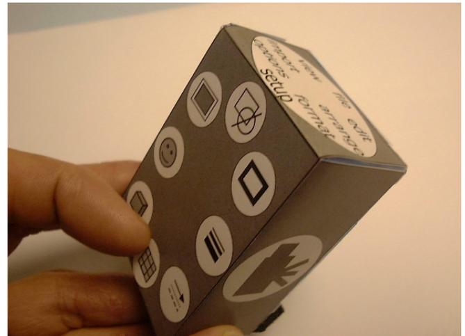
Figure 8: A ToolStone device with labels on each face. A (novice) user would be able to visually inspect available commands by physically turning the device.
